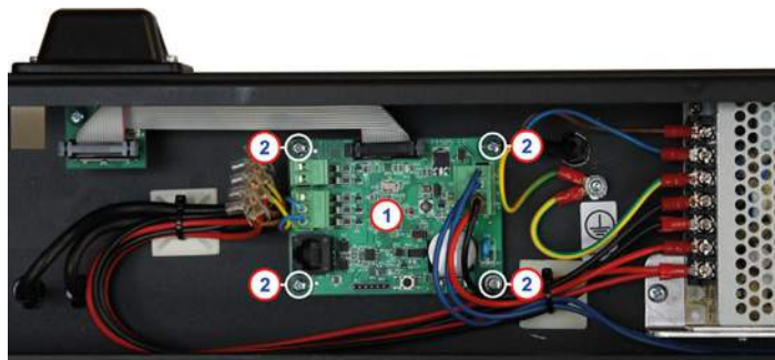
Fig. 8 Replacing a FC HUB board.
