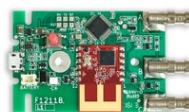
Art.897-32 ...F1211B electronic board for WF1-TRANSMITTER Spare part Size: 7.2x4.2x1.2cm. - Weight: 0.015kg.
