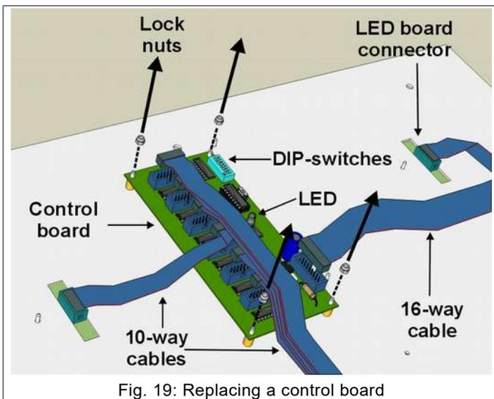
Fig. 19: Replacing a control board
