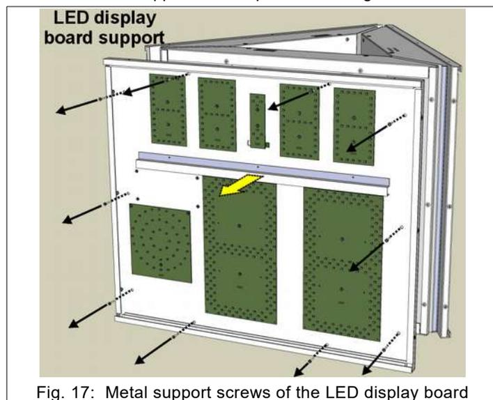
Fig. 17: Metal support screws of the LED display board
