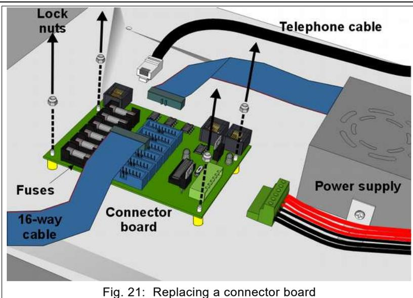
Fig. 21: Replacing a connector board
