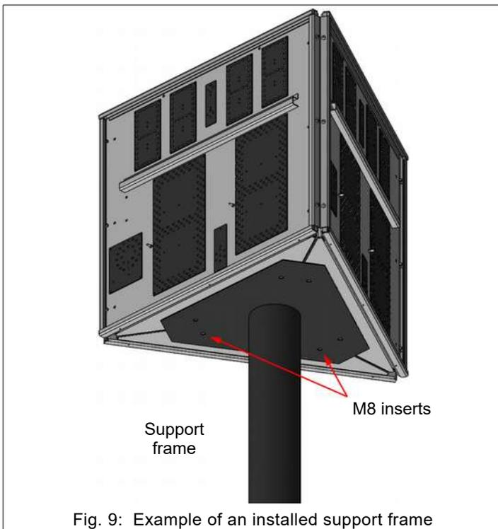
Fig. 9: Example of an installed support frame
