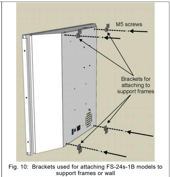
Fig. 10: Brackets used for attaching FS-24s-1B models to support frames or wall
