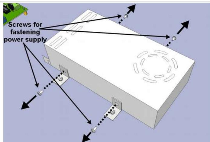
Fig. 22: Replacing the power supply unit
